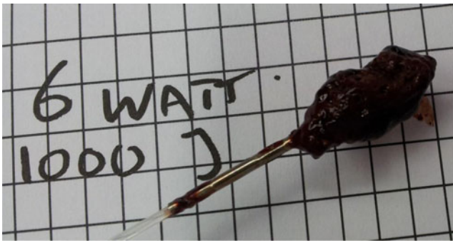
Fig. 3 Coagulum on a fiber tip held stationary in blood; the laser at 1,470 nm wavelength emitted 1,000 J of energy at a rate of 6 W
